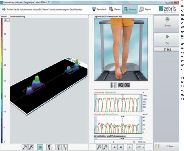
The display of all the measuring results is effected in real-time using commercially available PCs. A feedback control of the force on the extremities is thereby possible. The software provides a "Signal Viewer" in which all the recorded measuring variables are displayed in slow motion and completely synchronized. The allocation of the floor contacts to the left or right side of the body is carried out fully automatically by the evaluation software.
