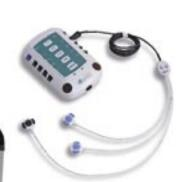
Besides the infrared interface, the cordless radio adapter has eight analog inputs, four digital inputs and an output for directly connecting a special USB adapter cable.
