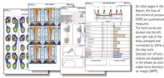
On other pages in the Report, the lines of the centers of pressure (COP) are automatically measured. The force curves are divided into the left and right side of the body, averaged and normalized to 100% of the step cycle. Selected roll-off procedures are displayed in the Viewer as color-
