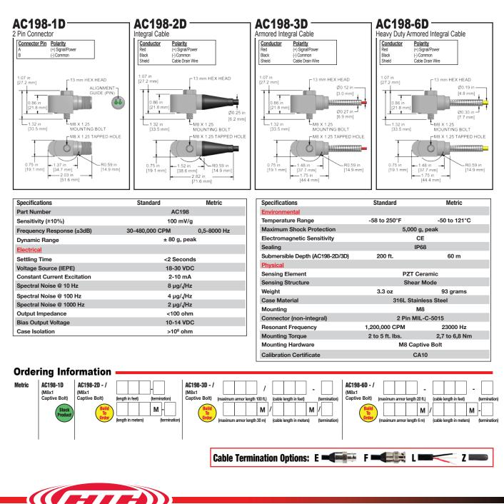
Accelerometers ATION SENSORS
