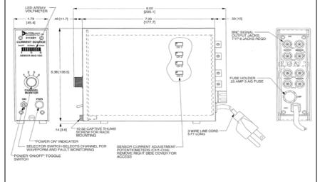
Units on the line drawing are in inches, units in brackets are in millimeters. Refer to 127-4114B1 for more information.
